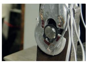
Tensile test on M16 fork using a break load of 150 kN. Photo: TU Munich
