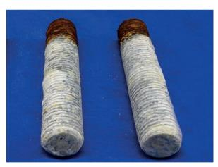
JACOB bar threads after 480 hours of salt spray test.
